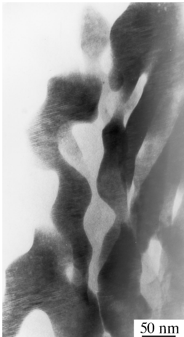
Fig. 14. YMAS matrix in composite P7, at Step 3 (see text). Low magnification TEM image. The lamellar eutectic microstructure deforms, and lamellar crystals tend to become spherical.
